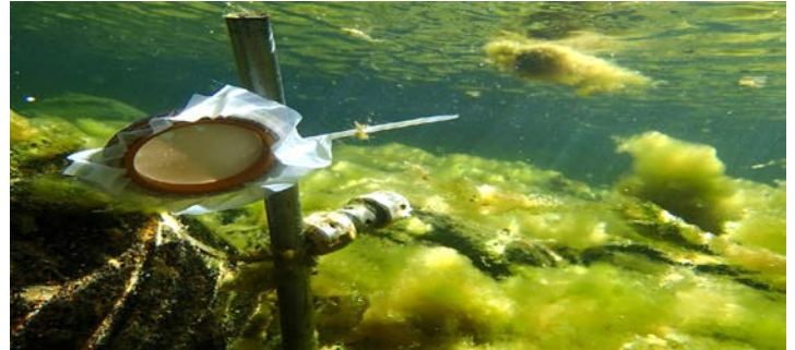
Solid Phase Adsorption Toxin Tracking (SPATT) bag in the Eel River. Photo Courtesy of Keith Bouma-Gregson
